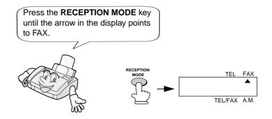
When the reception mode is set to FAX, the machine will automatically answer all calls on 2 rings and receive incoming faxes.
